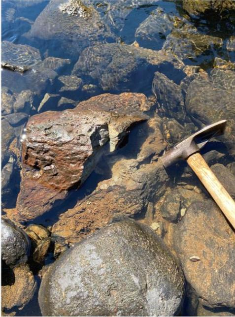
Angular, massive, banded pyrite-sphalerite-galena boulder discovered in brook in 2021 by Altius personnel. Sample 15902 of boulder assayed 18% Zn, 17.6% Pb, and 605 g/t Ag.
